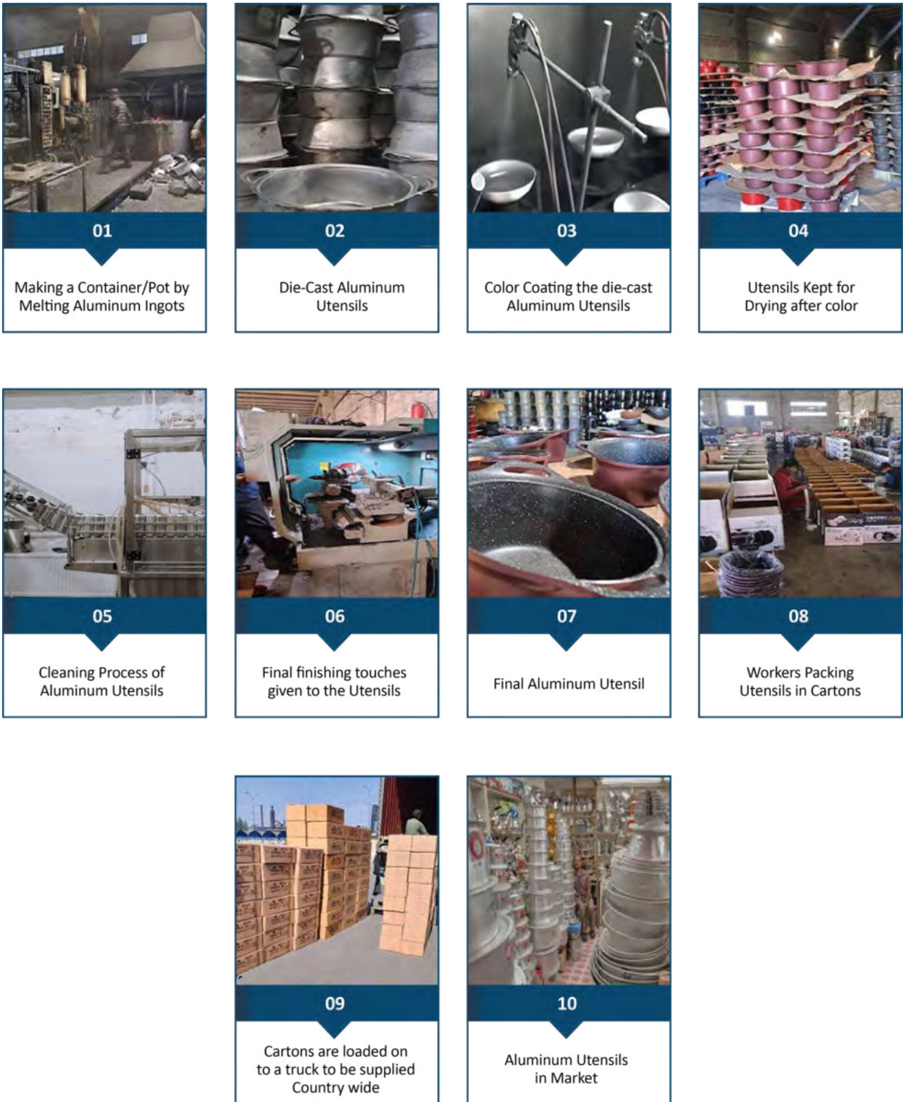
Figure 5.2: Die-Cast Aluminum Utensils Manufacturing Process
